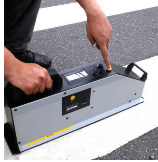
EASYLUX Retroreflectometer Easylux Minireflecto and Classic Retroreflectometers are the most advanced handheld solution for accurately measuring the retroreflectance of road markings, road studs and traffic signs.
